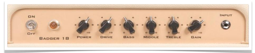
Saturated Lead: Power: 10, Drive: 4, Bass: 3, Middle: 6, Treble: 6, Gain: 8-10
